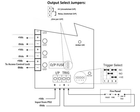
In the example above, power to the lock is removed when the 24Vdc signal from the Fire Alarm Panel is disconnected (*BS7273-4 Compliant*). When trigger select jumper set across 3 and 4.
