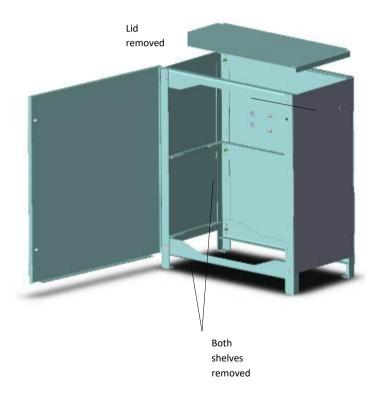
If not fitted, install the wall mounting bracket to the rear panel, using the provided 4 off M5 pan head screws and plain washers.
