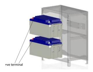
Fit positive and negative ends of 3m cable to the batteries as shown (crimped ring terminals):
