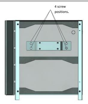
Position the case in its installation position. Spot through 4 fixing screw positions.
