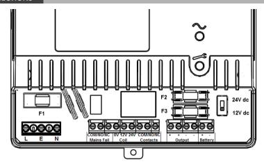
O/P +,+,-, -Dual (common) output connection to equipment to be powered
