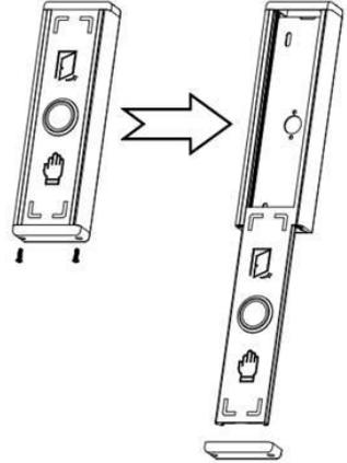
3. Fix the rear housing using suitable fixings and make suitable ground connection
