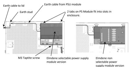
Step 2: Install earth cable from earth stud to lid.
