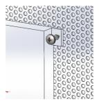
1. Align controller in suitable position in enclosure
